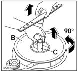
To take it out remove the spray arm by pulling it upward on one side, turn the column (C) anticlockwise by 90° and then slide out the filter.
